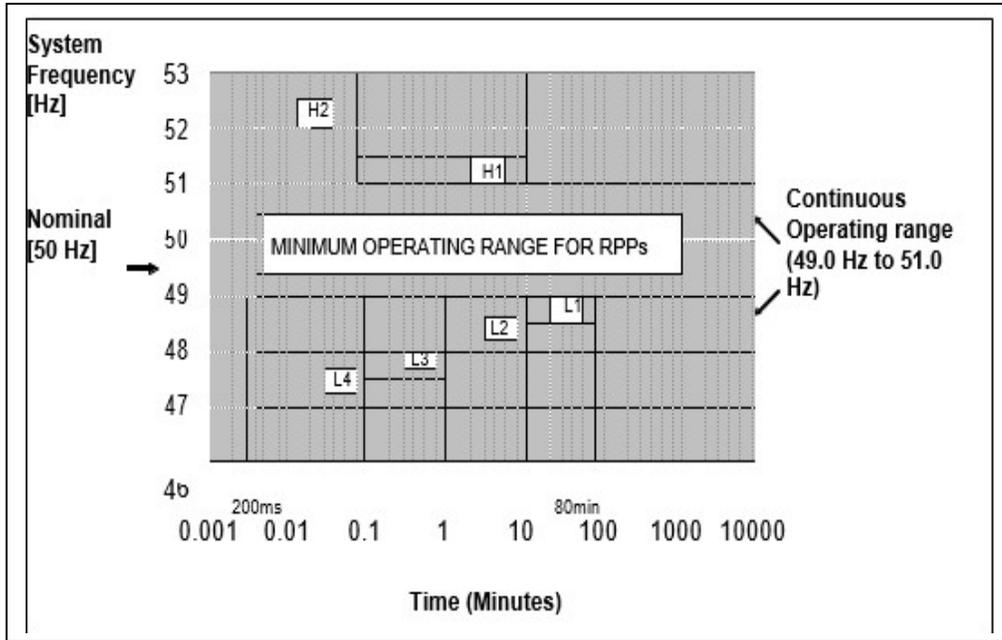
**Figure 1: Minimum frequency operating range for RPP (Cumulative over the life of the RPP)**
