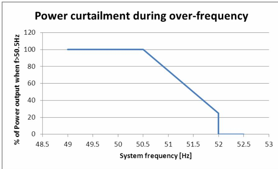
**Figure 6: Power curtailment during over-frequency for *RPPs***
