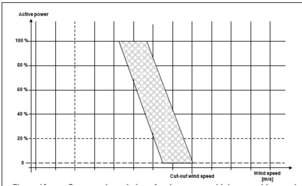
**Figure 16: Downward regulation of active power at high renewable speed**
