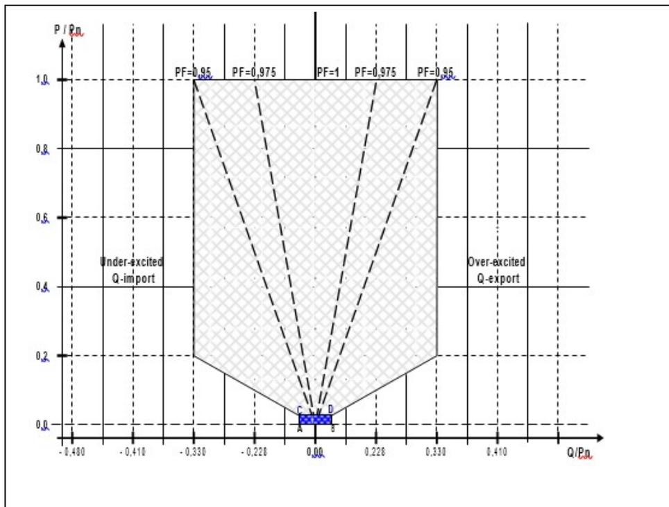
Figure 10b: Reactive power requirements for RPPs of category C (at nominal voltage at POC)
