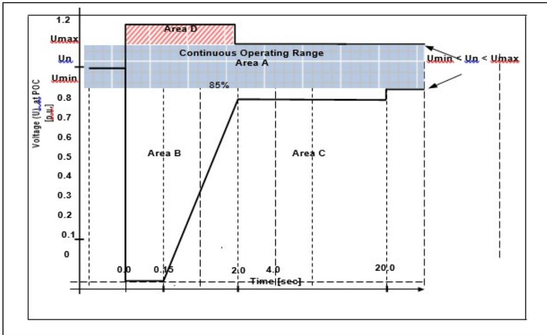
**Figure 4: Voltage Ride Through Capability for the RPPs of Category A3, B and C**
