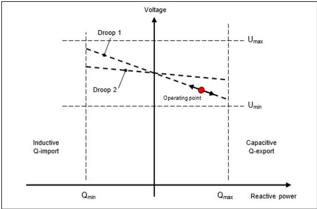
Figure 13: Voltage control for the RPP
