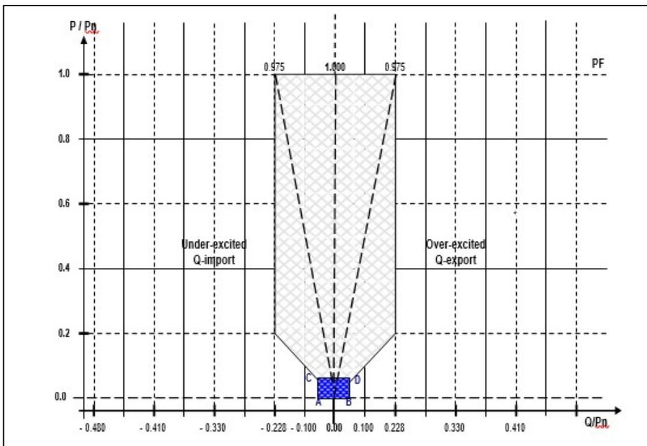
Figure 8b: Reactive power requirements for RPPs of category B (at nominal voltage at POC)
