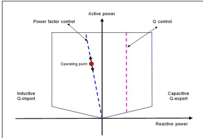
**Figure 12: Reactive power control functions for the RPP**
