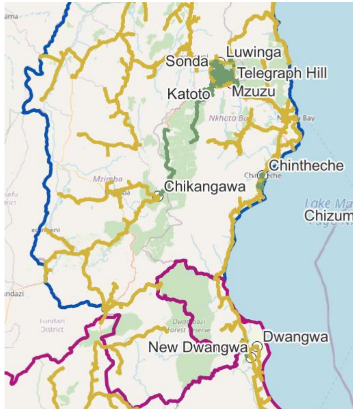
Figure 3.5.9: Downer part of the Northern region (33kV feeders are in brown – 11kV feeders are in green)
