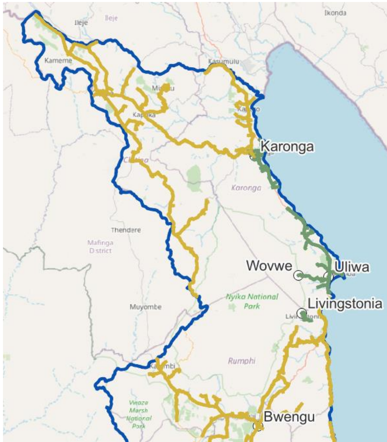
Figure 3.5.8: Upper part of the Northern region (33kV feeders are in brown – 11kV feeders are in green)
