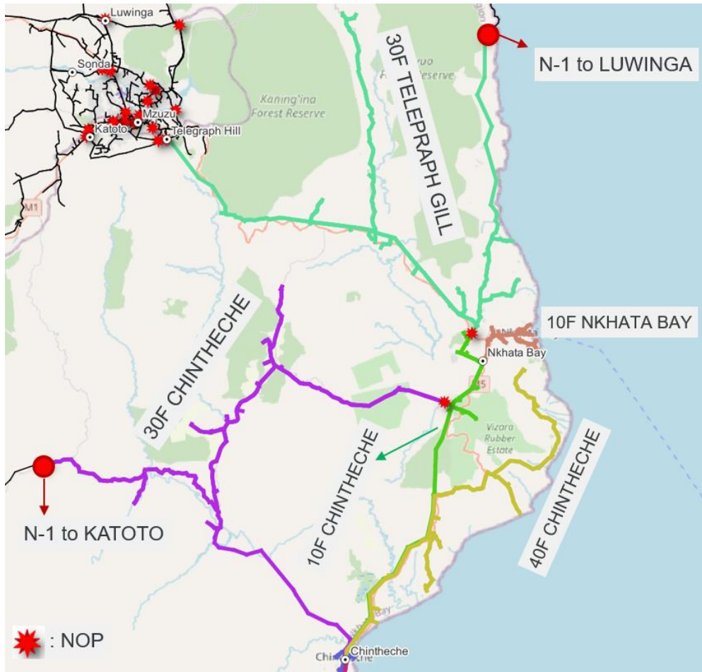
Figure 3.5.19: Rearrangement of 33kV feeder 10F CHINTHETCHE
