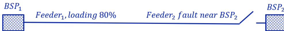
Figure 3.5.3: Illustration of the normal and contingency situation in case of a fault of the feeder near the BSP
