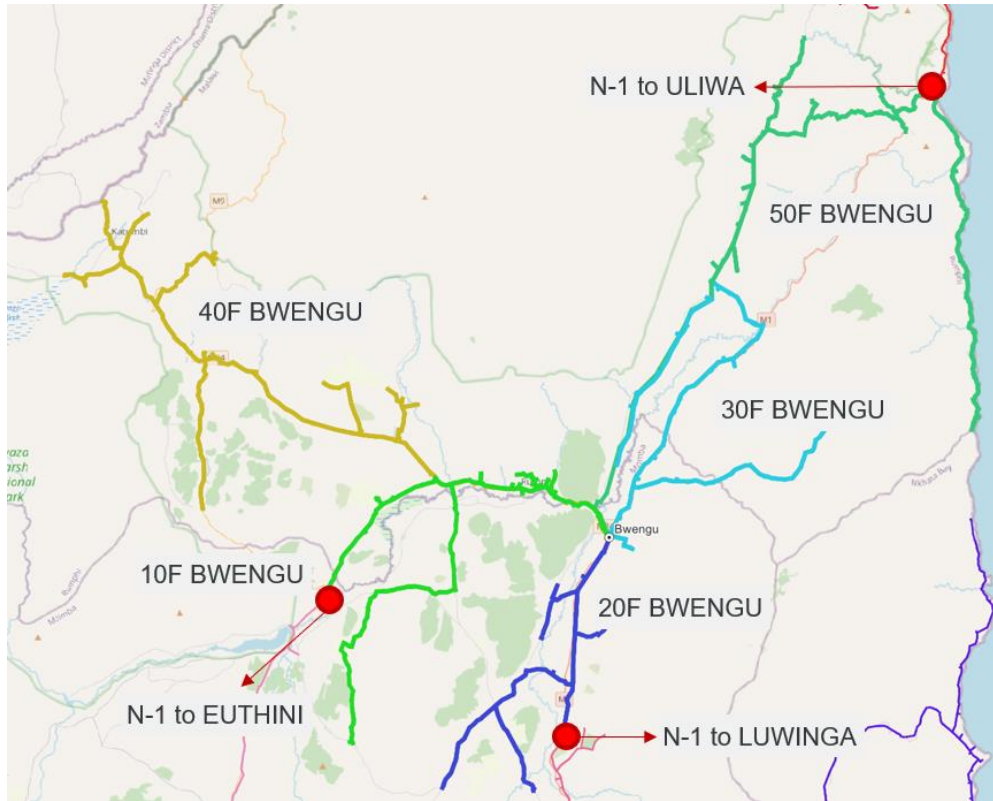
Figure 3.5.13: 33kV feeders leaving Bwengu station
